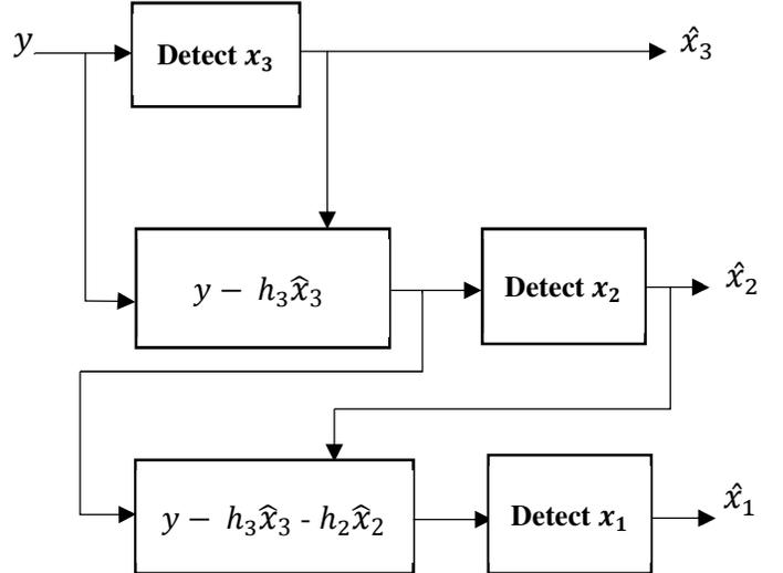
Fig. 2. Illustration of SIC detection of the signals at the base station with three users.
